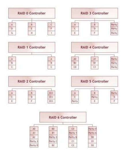
Also known as striping, RAID 0 uses any number of drives. Data is written sequentially by sector or block across the drives. This provides high read and write performance because many operations can be performed simultaneously, even when a sequential block of information is being processed. The downside is the lack of redundancy. Striping is commonly combined with other RAID architectures to provide high performance and
